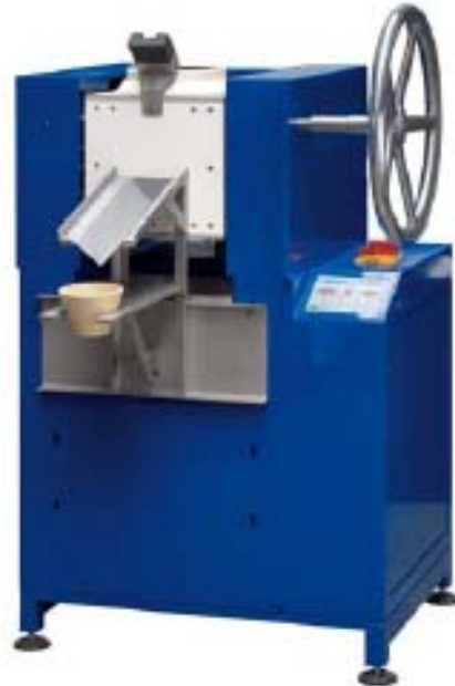
Version with tilting wheel, holder for shell moulds and spout on crucible
